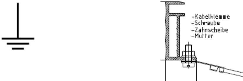
Figure 9: Equipotential bonding symbol and design
