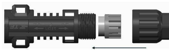
Figure 5 Connector Housing Components
